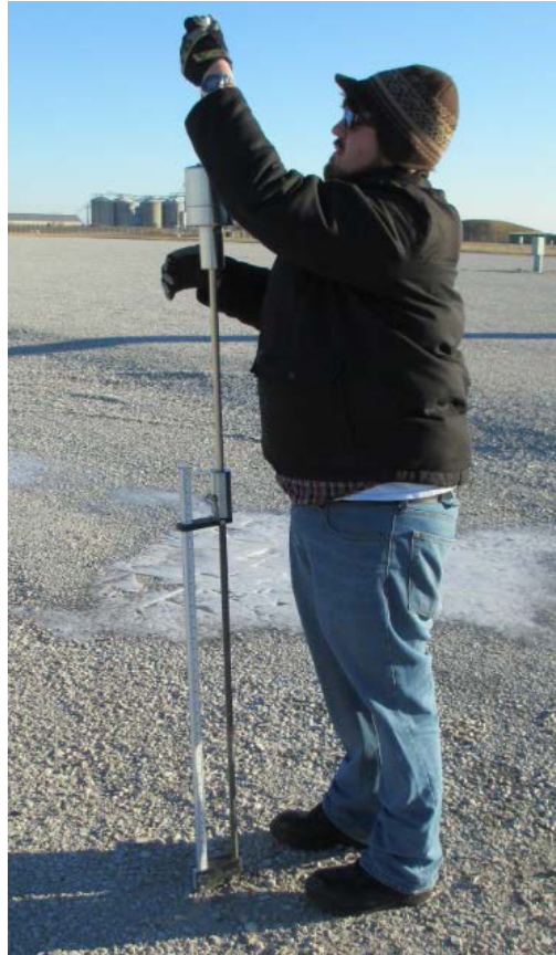
Figure 38. In situ DCP test
