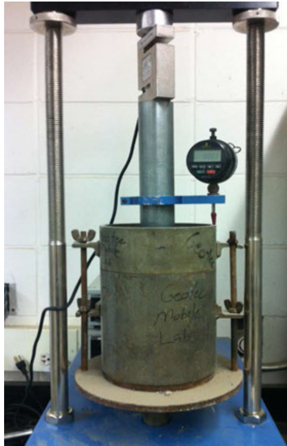
Figure 27. CBR test device
