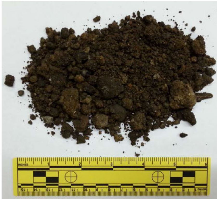
Figure 43. Subgrade from the Boone County Test Sections site
