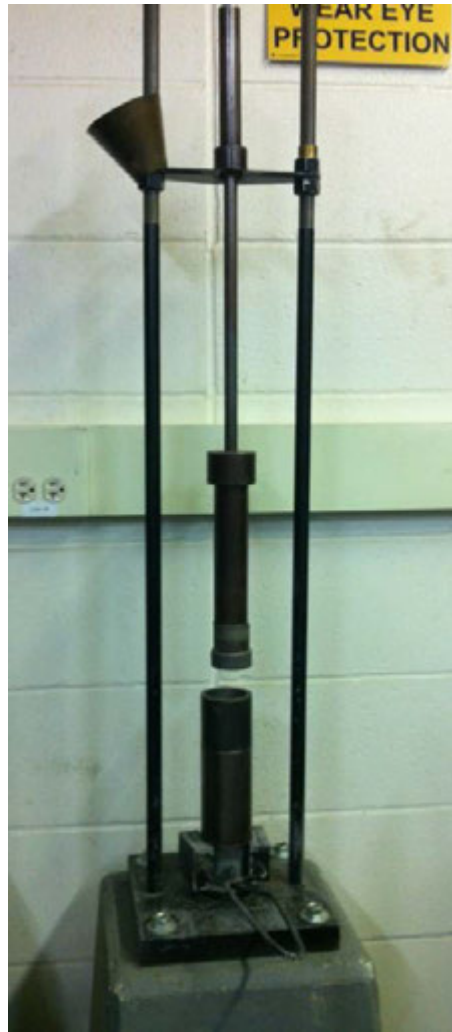
Figure 25. 2-in. x 2-in. compaction test
