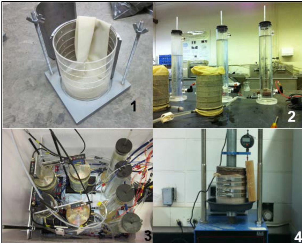
Figure 8. Laboratory freeze-thaw test steps showing (1) sample remolding; (2) fully saturation; (3) freeze-thaw process; (4) CBR test
