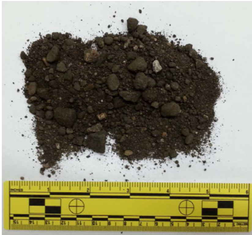
Figure 40. Recycled subbase from the Boone County Test Sections site
