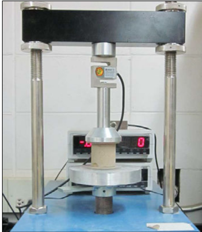
Figure 26. 2-in. x 2-in unconfined compressive strength test
