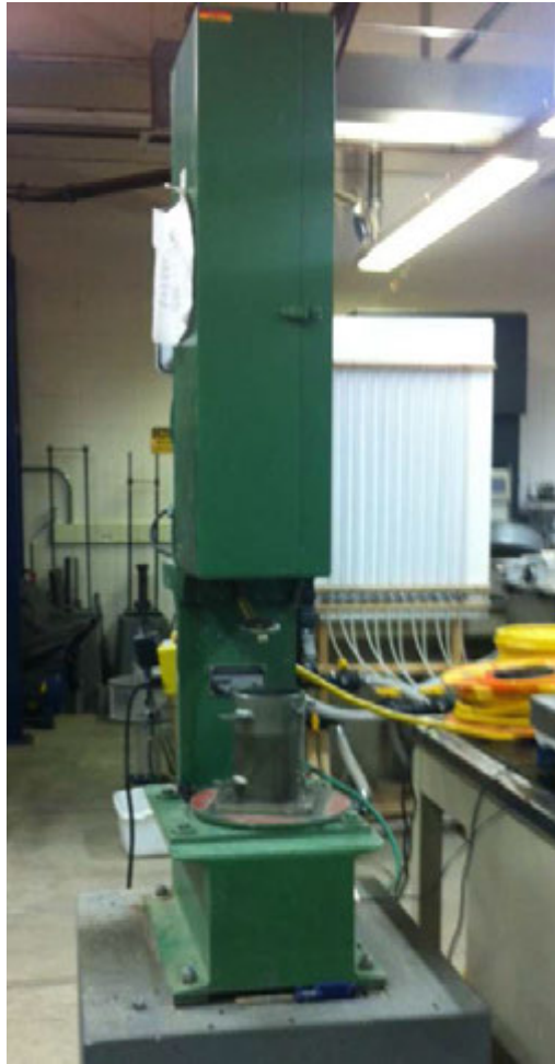
Figure 24. Standard Proctor compaction test
