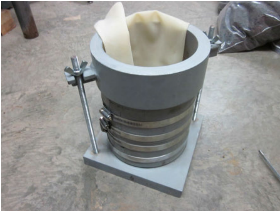
11. Stretch the membrane around the collar.
