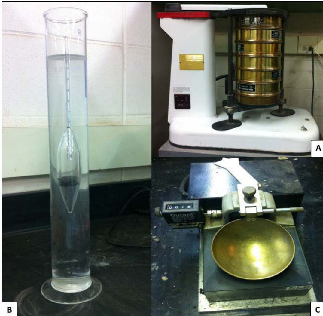
Figure 23. Soil classification tests showing (a) Sieve test; (b) Hydrometer test; (c) Atterberg limits test.
