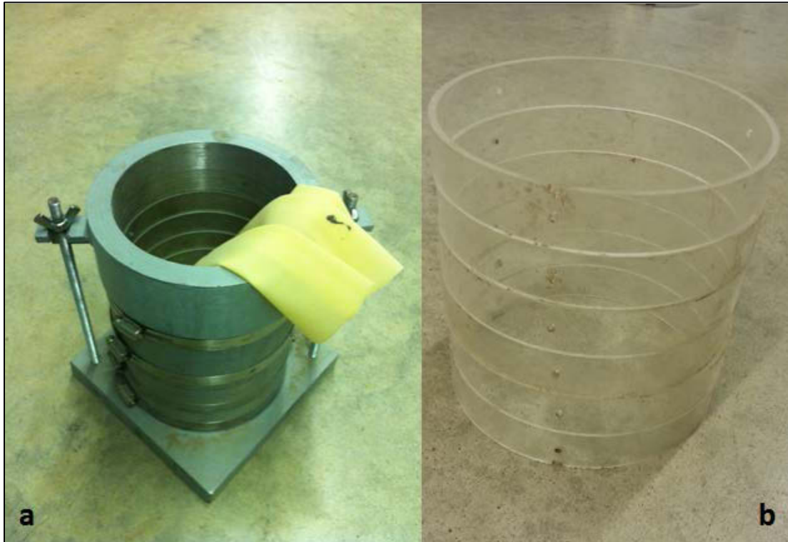
Figure 29. Sample assembly showing (a). Sample setup; (b). Six acrylic rings
