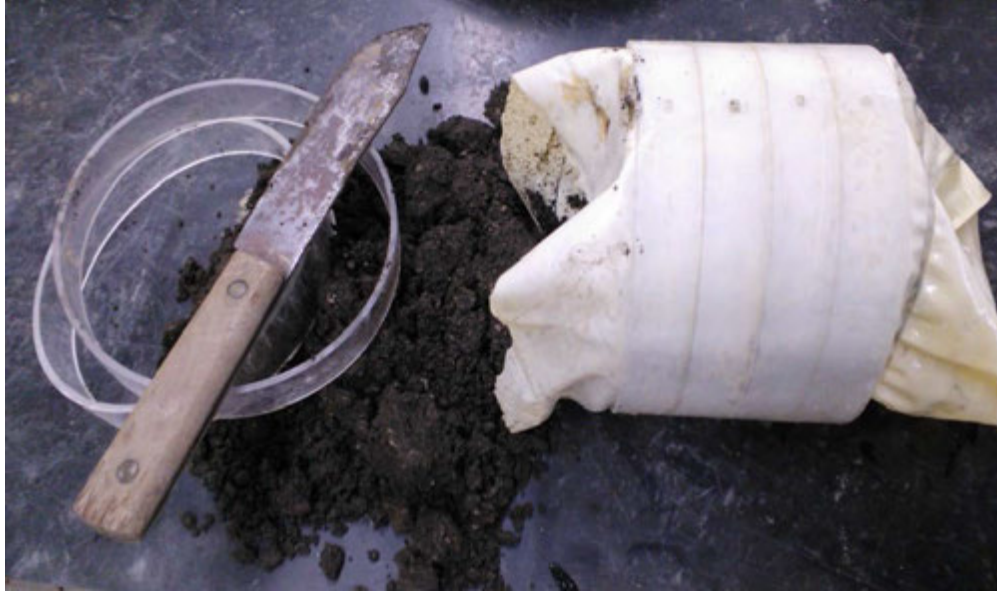
Figure 37. Cut the sample into six layers
