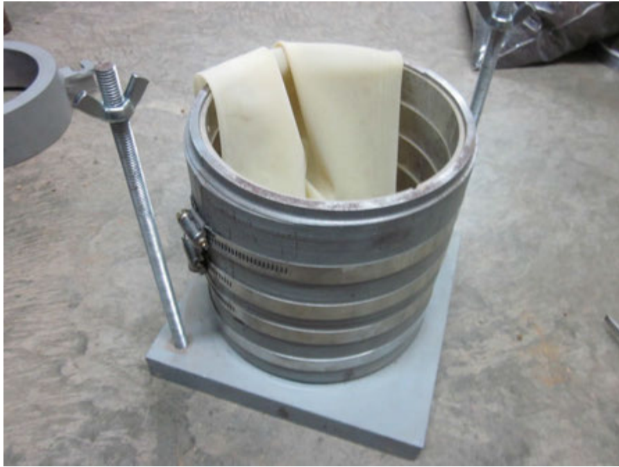
10. Place the collar on the mold and tighten the wing nuts
